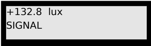
'SIGNAL': This message is displayed continuously in the 'mode of operation' register (lower left corner of the LCD) after the 'SIGNAL' button has been pressed, indicating that the instrument is in constant wave measurement mode.
