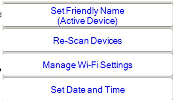
3S. Re-Scan Devices: Scrolls through all com ports to look for new or additional devices and/or device names and connects to them. (applies USB all or USB first based on settings in 3O. Discovery Type) After Re-Scan devices use the Select Active Device to verify all devices are listed in the drop down menu.
