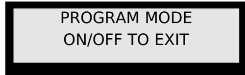
To enter 'PROGRAM' mode, begin with the ILT1400 turned on and a detector plugged in. Next, press the 'OFF' button and within 1 second press the 'ZERO' button. The LCD message 'PROGRAM MODE', 'ON/OFF TO EXIT' will appear. You can get out of 'PROGRAM' mode at any time by pressing the 'ON/OFF' button. When in 'PROGRAM' mode, the push buttons assume alternate functions:
