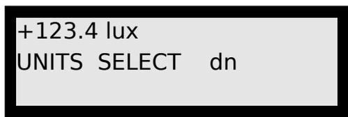
Press the ‘MENU’ (ZERO) button to scroll to the ‘UNITS SELECTION’ menu screen. Use the ‘SELECT’ (SIGNAL) button to choose ‘UP’ or ‘dn’, changing the direction that you scroll in the list of units. Press the ‘INCREMENT’ (INTEGRATE) button to scroll to the next
