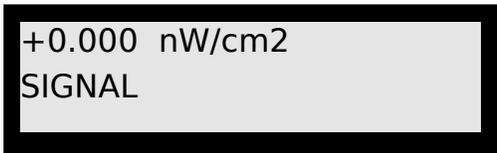
'ZEROING': This message is displayed temporarily in the 'mode of operation' register (lower left corner of the LCD) after the 'ZERO' button has been pressed, measuring the present light level and subsequently returning to 'SIGNAL' mode while subtracting this ambient light from future readings.
