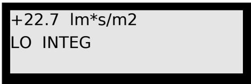
'HI INTEG' or 'LO INTEG': One of these messages is displayed continuously in the 'mode of operation' register (lower left corner of the LCD) after the 'INTEGRATE' button has been pressed, indicating that the instrument is in light integration mode. Press the 'INTEGRATE' button twice within one second to alternate between the 'HI' and 'LO' integration ranges. Press the integrate button once to reset the integral register in that mode to zero.
