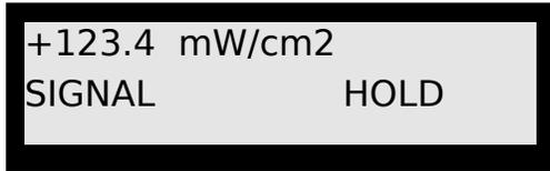
Pressing the 'HOLD' button while in 'SIGNAL' mode will freeze the last reading on the display, and the word 'HOLD' will blink in the status register of the LCD. To resume constant wave measurement, simply press the 'SIGNAL' button or toggle the 'HOLD' button again and the instrument will return to 'SIGNAL' mode (with the same zero level as before).
