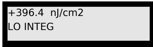
In 'LO INTEG' mode, the range for an incoming signal is limited to the bottom 4.5 decades of the measurement range of the detector, overlapping with the 'HI INTEG' range by 2 decades. The measurement range in 'LO INTEG' mode is from 10 picoAmps to 400 nanoAmps. The added gain (256 times) and sensitivity of this mode are provided at the expense of a narrower dynamic range, and are limited by increased noise on the low end.
