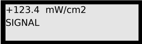
The ILT1400 uses a two line, thirty-two (32) character “Supertwist” Liquid Crystal Display (see above) to portray numerical data, units, mode of operation, and instrument status alphanumerically in bit-mapped graphics. If the instrument is turned on without a detector plugged in, the display will instruct the user to ‘SHUT POWER OFF’, ‘PLUG DETECTOR IN’, in order to properly initialize the ILT1400 system.
