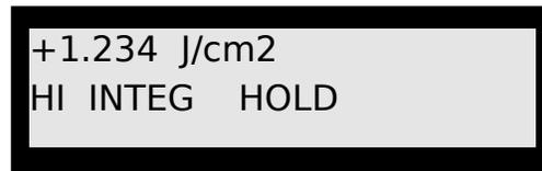
'HOLD': This message will blink in the 'status' register (lower right corner of the LCD) after the 'HOLD' button has been pressed, activating the 'HOLD' feature. The most recent reading will be frozen on the data display. To remove the 'HOLD' status, toggle the 'HOLD' button again or hit a function key ('SIGNAL', 'INTEGRATE', or 'ZERO') to select a new mode of operation.
