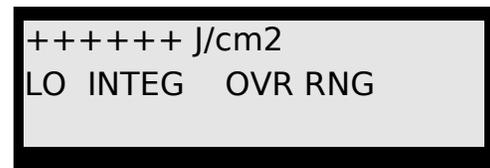
'OVR RNG': This message will blink in the 'status' register (lower right corner of the LCD) when the input detector signal exceeds the measurement range of the system. In addition, plus signs take the place of numerals in the data display, so that the top line will read '++++++ W/cm2'. If the signal over ranges in 'LO INTEG' mode, hit the 'INTEGRATE' button twice within one second to switch to 'HI INTEG' mode and a higher signal range.
