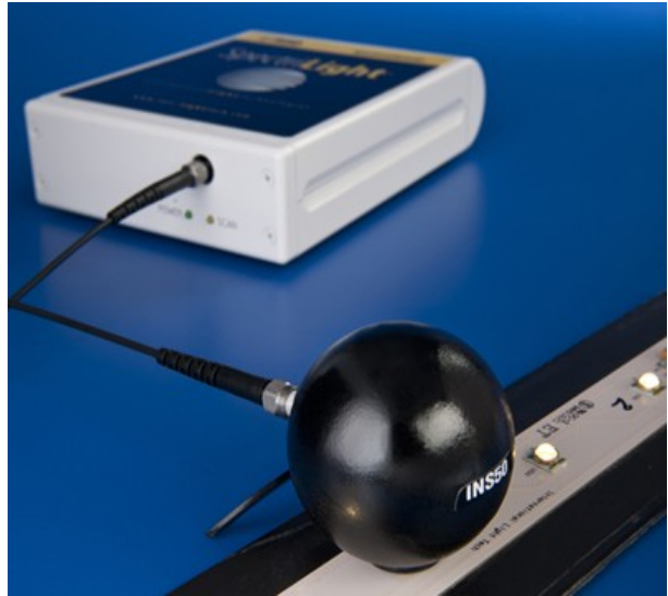
INS50 2" Sphere and ILT950 Spectroradiometer for Measuring LED's
